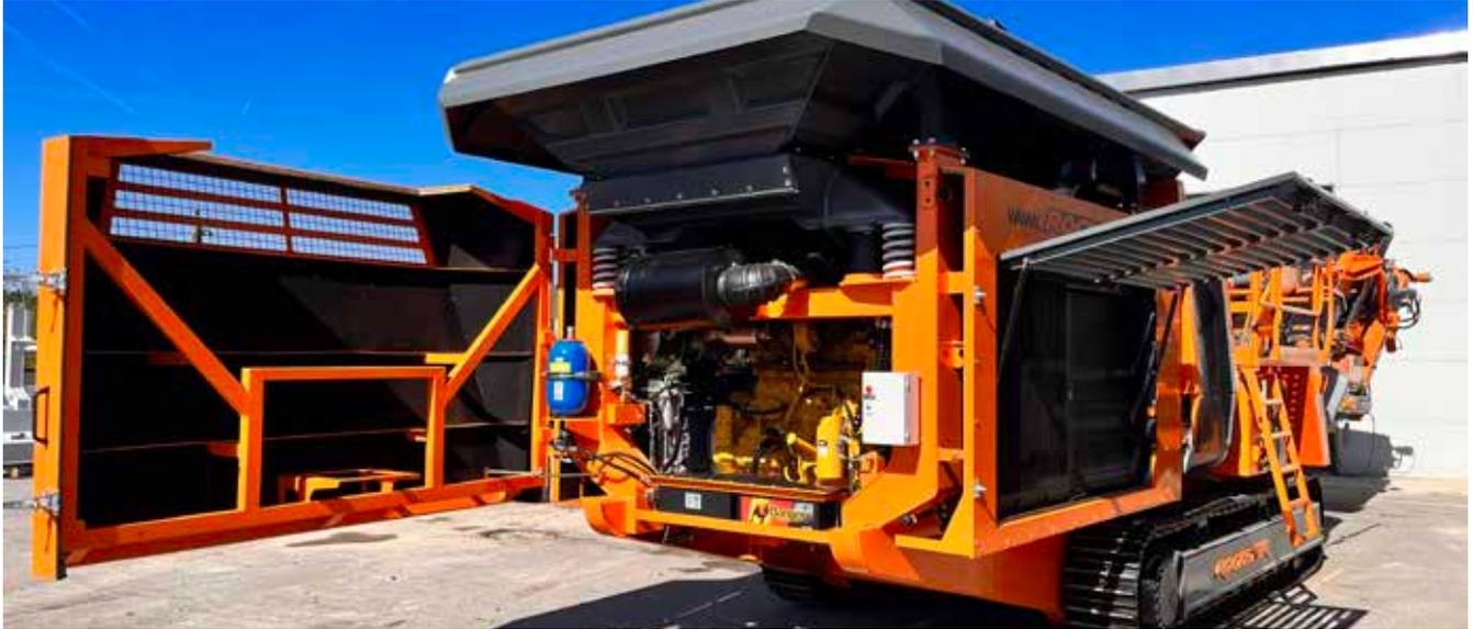
Large covers enable optimal accessibility when it comes to service and maintenance. Furthermore they ensure optimal ventilation of the drive-unit and the cooler. It makes it a dream for every service technician when it comes to service and maintenance.
