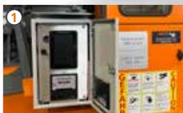
1 Belt weigh scale incl. printer
