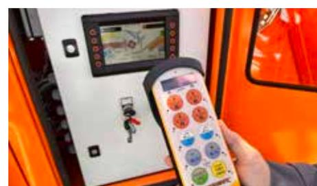
Intuitive easy-to-use central machine control unit with a radio remote control.
