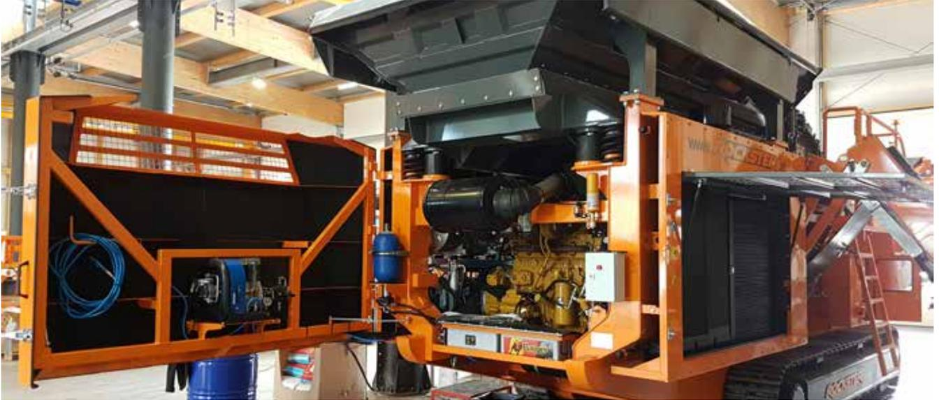
Large covers enable optimal accessibility when it comes to service and maintenance. Furthermore they ensure optimal ventilation of the drive-unit and the cooler.
