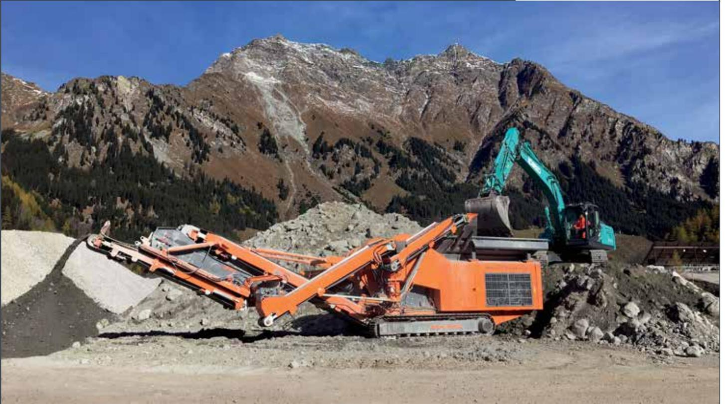
*By using the patented Rockster DUPLEX-System with jaw and impact crusher on one basic machine, the Casaccia gravel quarry at the base of the 'Maloja Pass' in Graubünden (Switzerland) can quickly and efficiently meet the diverse requirements of its customers.*
