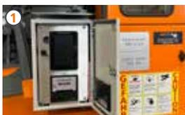
1 Belt weigh scale incl. printer
