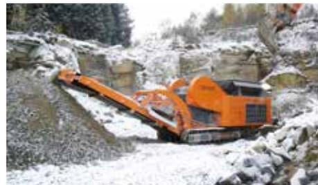
Compact, mobile & easily moved around the quarry. Ideal crusher for hard rock.
