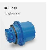
Each track is driven by a 2-speed automatic shifting travel motor, equipped with multiple discs and spring-locked and hydraulic-released brake. The unchallengeable traveling speed can reach up to 3.2 mi/h.
